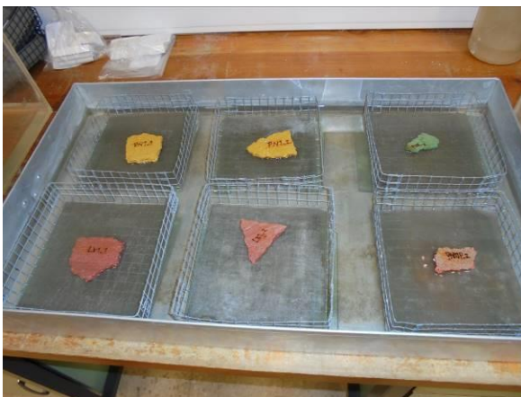
Figure 6. Physical and mechanical testing: a) Water absorption by capillarity; b) Compressive strength
