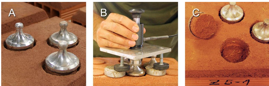
Figure 2. Pull-off test: A - Metallic devices glued to the plaster specimens; B – Pull-off equipment perpendicular to the specimen being tested; C – specimen after cohesive rupture
