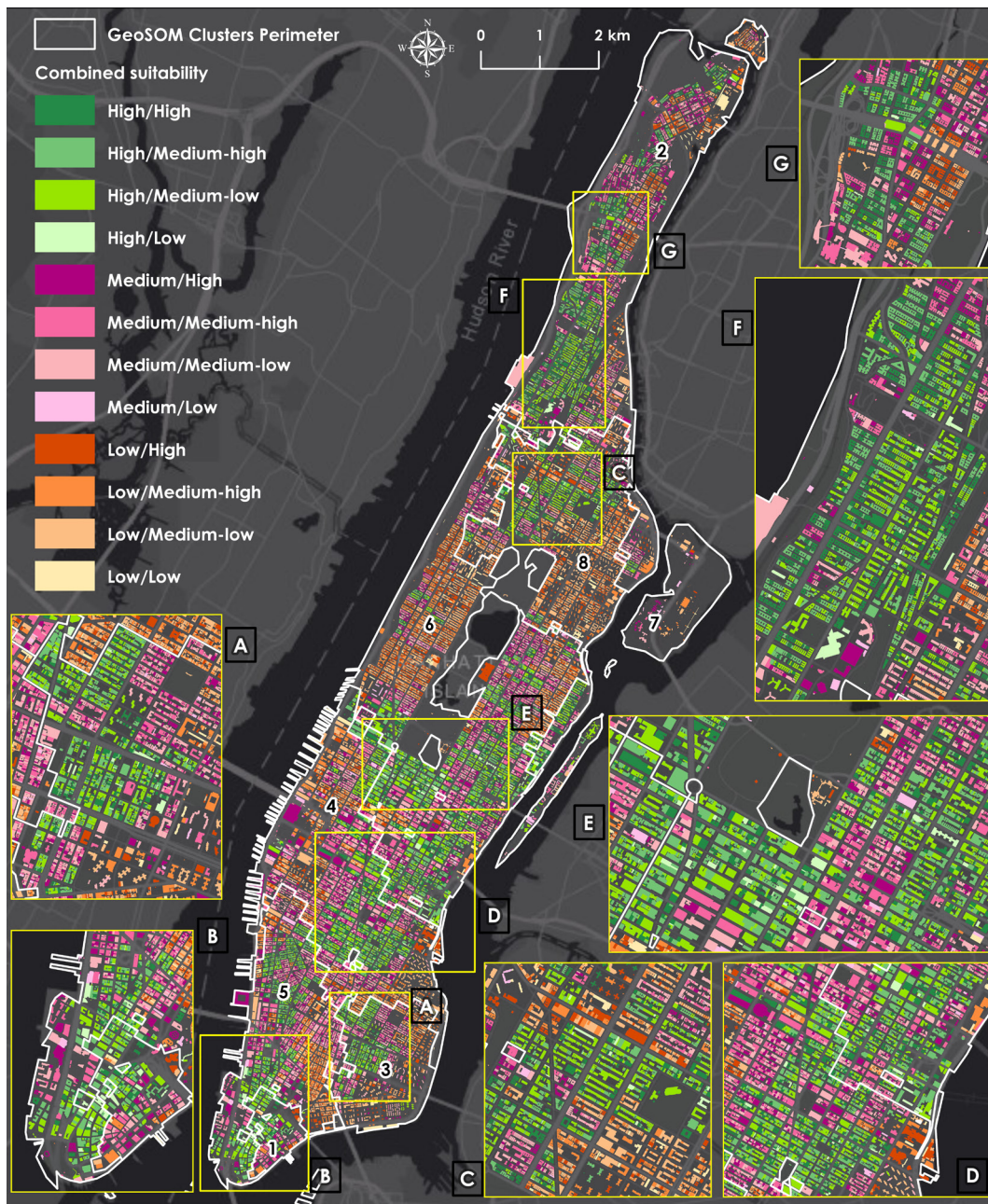
Figure 48. Combined suitability taking the criteria of place and flatness of the main surface on the roofs
