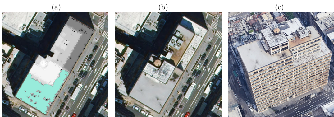
Figure 39. Roof 2 (a) Lidar image with main surface, (b) Satellite image, (c) 3D scene
