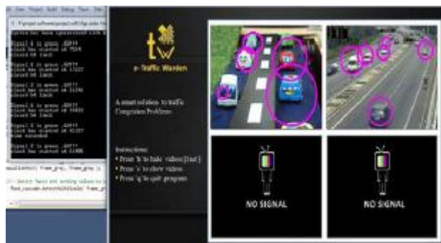
Figure 2.6: Application of the algorithm for the recognition of vehicles in OpenCV [23].
