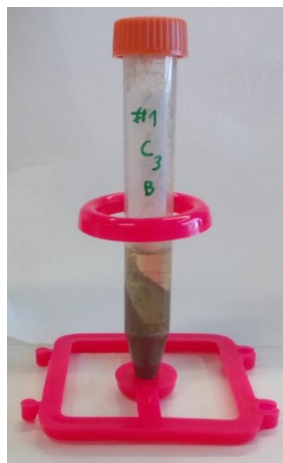
Figure 3.4 Sample in a falcon tube before collecting the supernatant.
