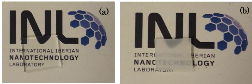
Figure 3.1: Developed phantoms - (a) one-layer clear PDMS (b) one-layer PDMS incorporated with TiO 2
