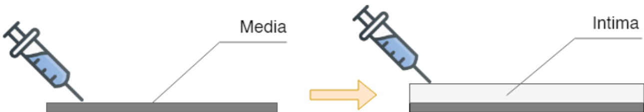
Figure 3.2: Schematic of double layer phantom shaping and the two replicated layers
