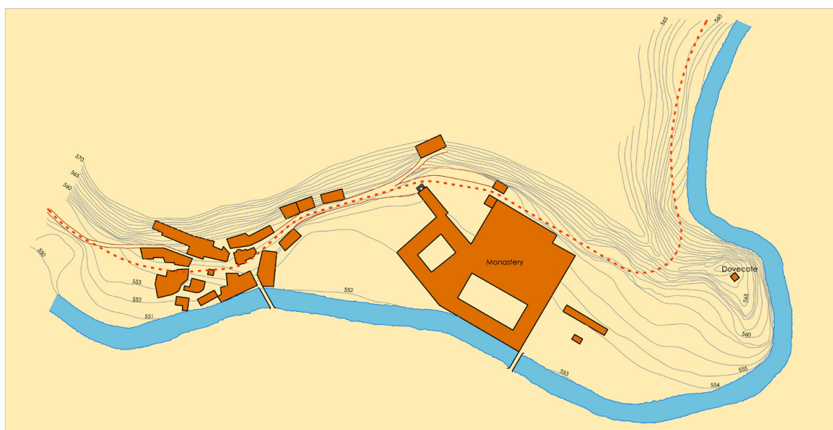
Fig. 3. Project of the road that passes through Samos village, scale 1:1,000, 1890. The new road is a red dashed line Source: Drawing by the author from the original map, which is preserved at AHPLu
