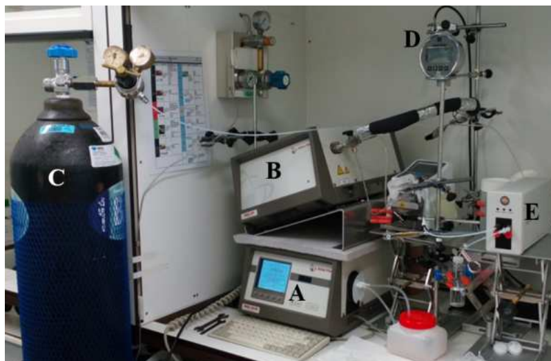
Figure II.8 IPQ's setup assembled to measure fluids' density for pressures up to 10 bar. Legend: oscillation-type density meters from Anton Paar: A – DMA 5000 (for density measurements at atmospheric pressure); B – DMA HP (for density measurements up to 600 bar); C – pressure generator – nitrogen gas cylinder; D – pressure gauge (IPI300 from Ametek JOFRA); E – membrane degasser (Degasi GPC from, Biotech).
