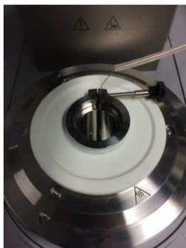
Figure III.31 Platinum resistance thermometer, connected to a data acquisition unit 34970A (Agilent), placed inside the hole of the cup of the coaxial-cylinder (CC27) measuring geometry, in the MCR 502 (Anton Paar) rheometer.
