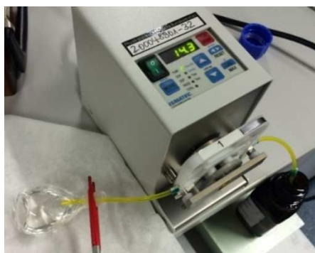
Figure III.24 Assembling used for filling the Gay-Lussac pycnometer with the non-Newtonian liquids tested by means of a peristaltic pump (ISM831C, ISMATEC) with a Tygon HC F-4040-A tube from ISMATEC.
