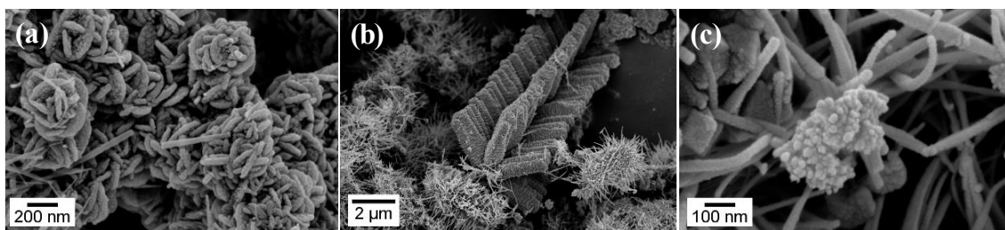
Figure 2.21. Mixture of nanostructures obtained with \text{ZnCl}_2 precursor with a \text{H}_2\text{O} :EDA volume ratio of 6:9: (a) \text{Zn}_2\text{SnO}_4 octahedrons comprised by nanoplates, (b) ZnO columnar nanoplatelets and (c) \text{SnO}_2 nanoparticles.
