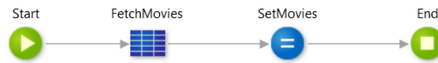
Figure 5.1: An example of an Action content. These four elements that constitute this action are called action nodes.
