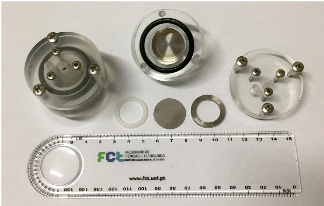
Fig.A6 1 - Assembled and disassembled bioreactors used in cellular culture assays
