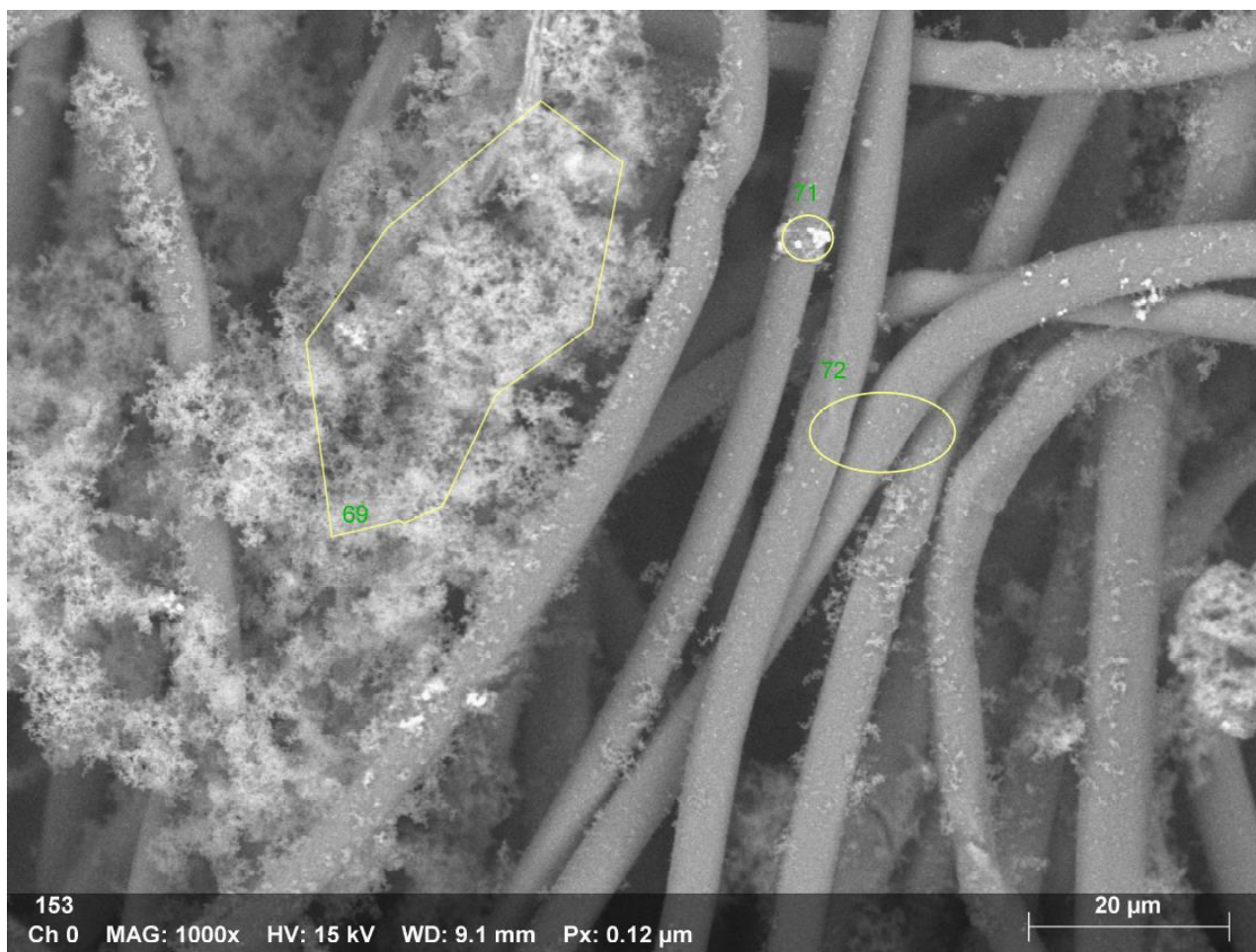
Figure B0. 2-SEM image of felt-PPy and identified clusters.
