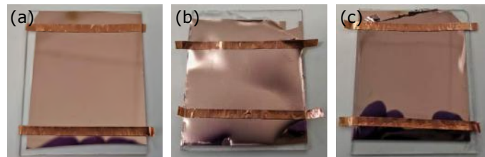
Figure A.2: Samples with deposited Cu and copper tape. (a) Cu deposited on Glass; (b) Cu deposited on PDMS with Parylene C; (c) Cu deposited on PDMS. Cu was deposited by E-beam on all samples.
