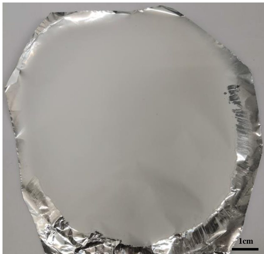
Figure 6 – Electrospun P(VDF-co-TrFE) membrane
