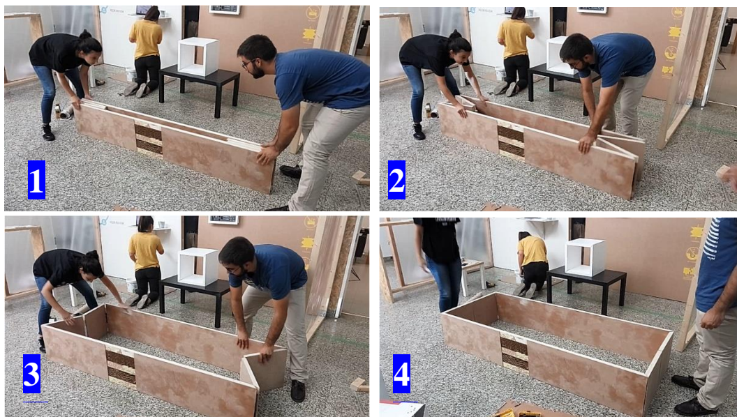
Fig. 36 – PAX cabinet prototype with LÄNK Technology (sourced from team)
