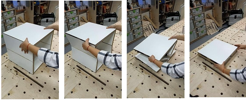
Fig. 35 – Folding movement of the Part X prototype (sourced from team)
