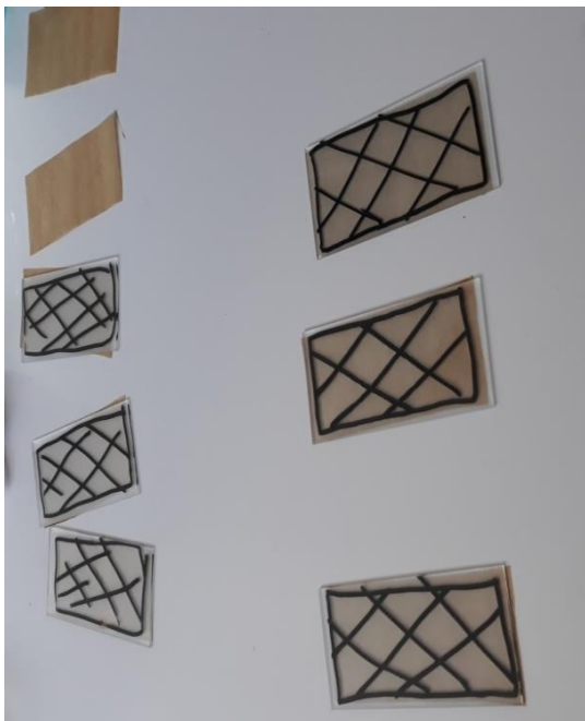
Figure 21: Marked definitive glass slide for polishing.
