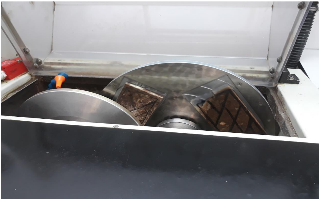
Figure 25: Polishing the sample surface.
