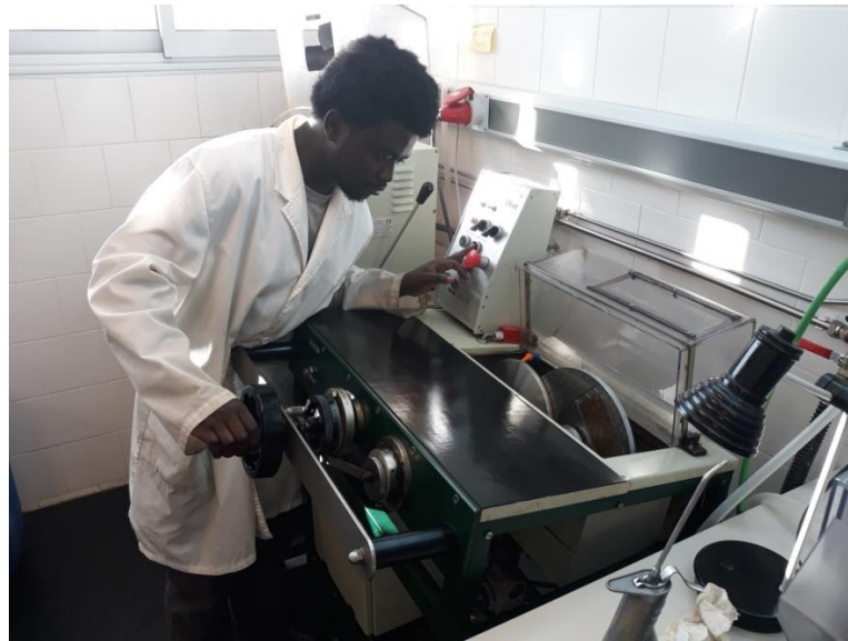
Figure 32: Polishing the samples to correct thickness.
