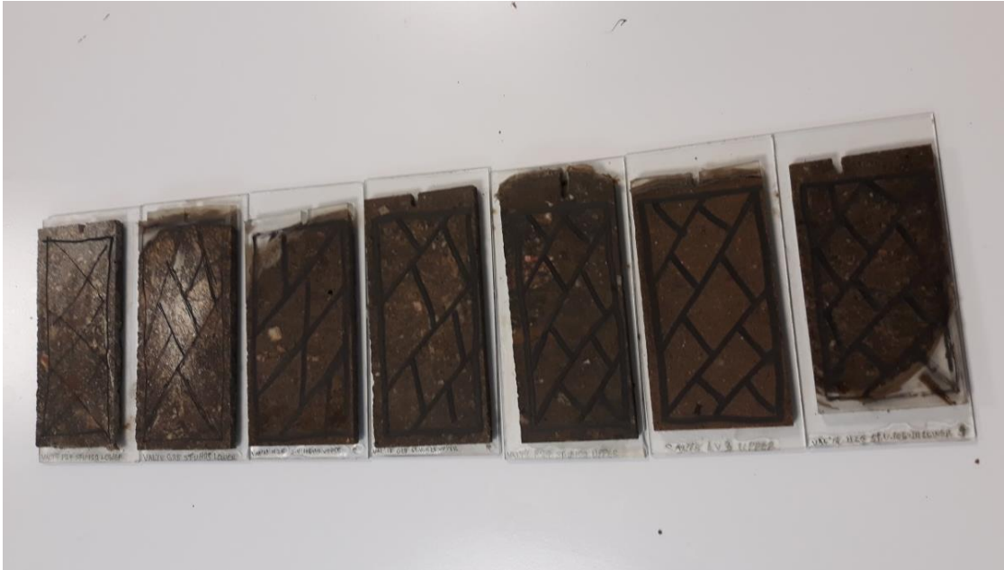
Figure 24: Marked surface of the sample for polishing.
