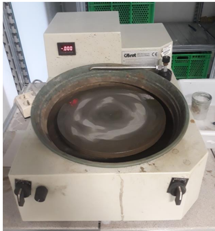
Figure 18: Glass grinding wheel for the glass slide preparation.
