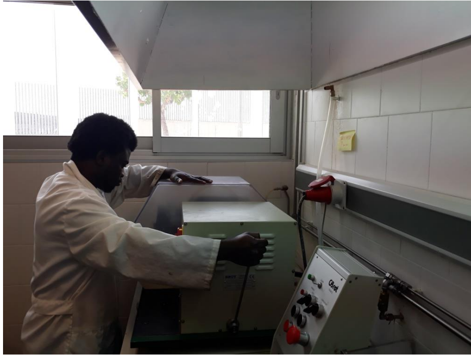
Figure 23: Cutting the first chip off the glued sample.
