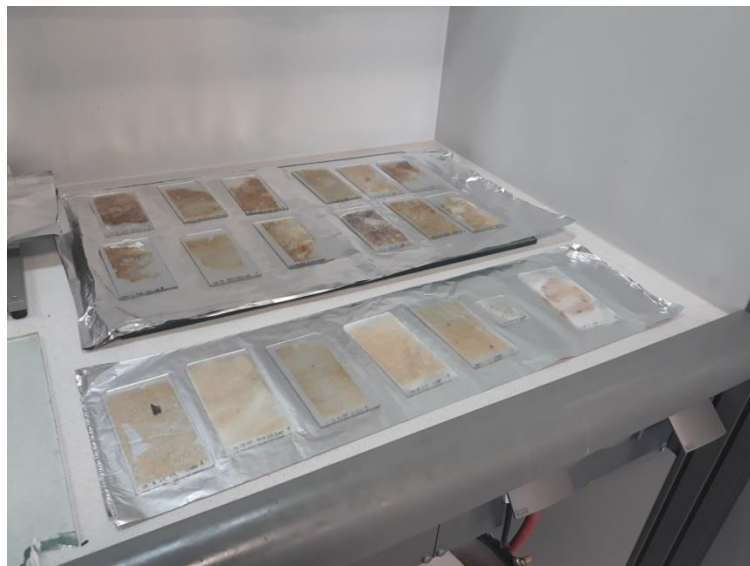
Figure 33: Thin section of 30 microns with a cover slip ready for microscopic observation
