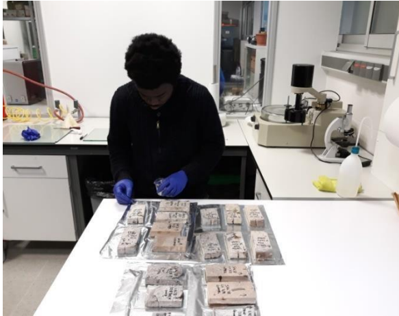
Figure 19: Applying epoxy to glue the samples.
