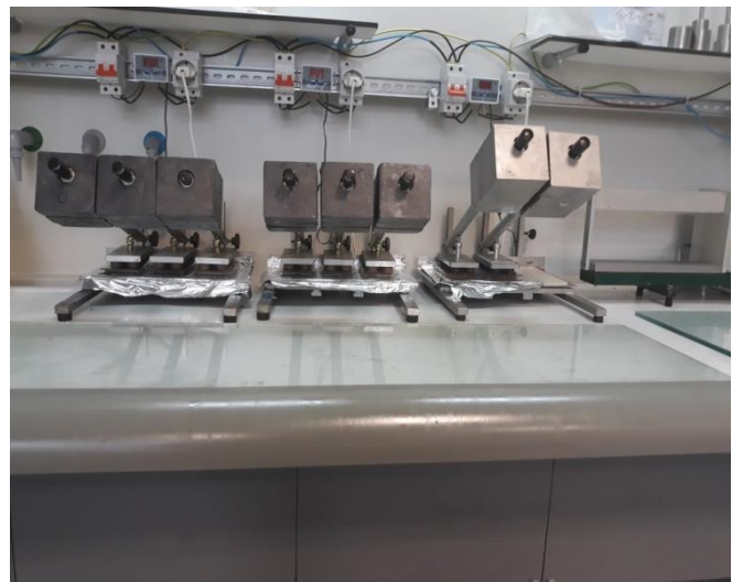
Figure 28: Glue samples properly to the glass slide.
