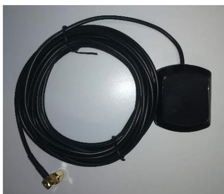
Figura 37 – Antena GPS do Stratio Databox (Stratio).
