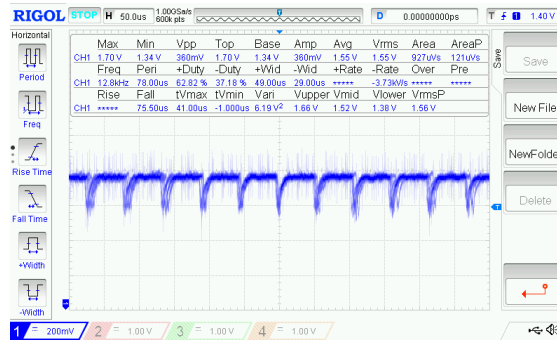
Figure 9.21: Receiver's signal conditioning board average voltage
