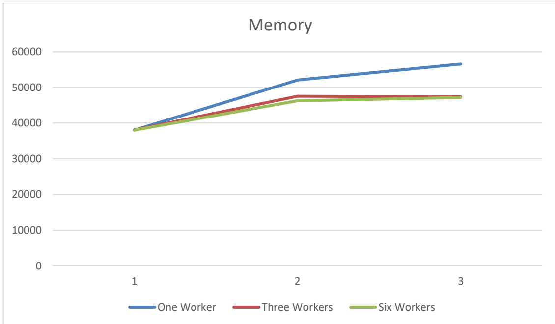
Figure 64 Local deployment standalone app memory usage
