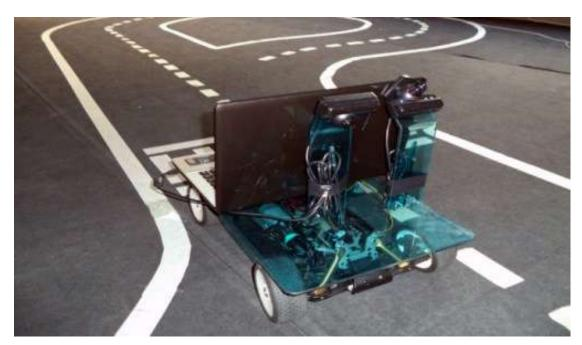
Figure 2.7: N3E GT Robotic platform - Polytechnic Institute of Leiria
