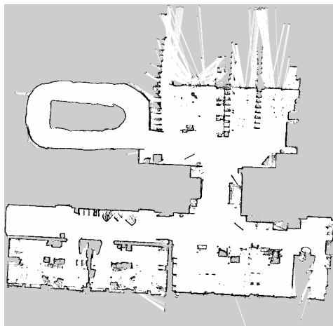
Figure 6.3: Generated Map from Hector SLAM of the Undergrad Lab Area at CISTER with a 0.03 resolution.
