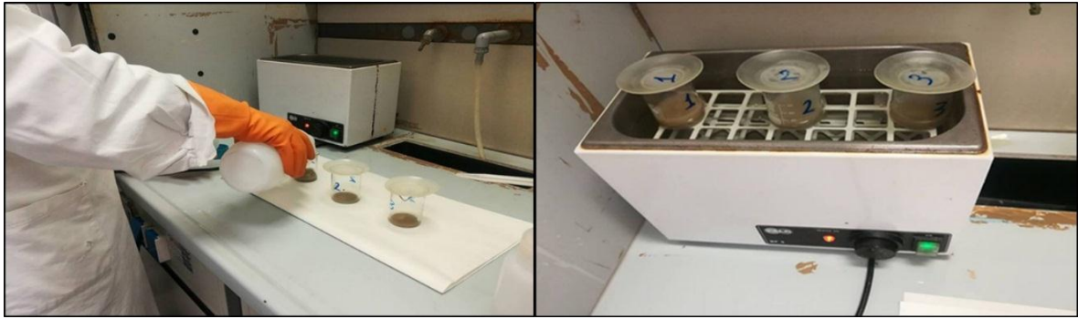
Figure 16: Processes of removing salts soluble in hydrochloric acid (HCl, 7%), and samples in water bath.
