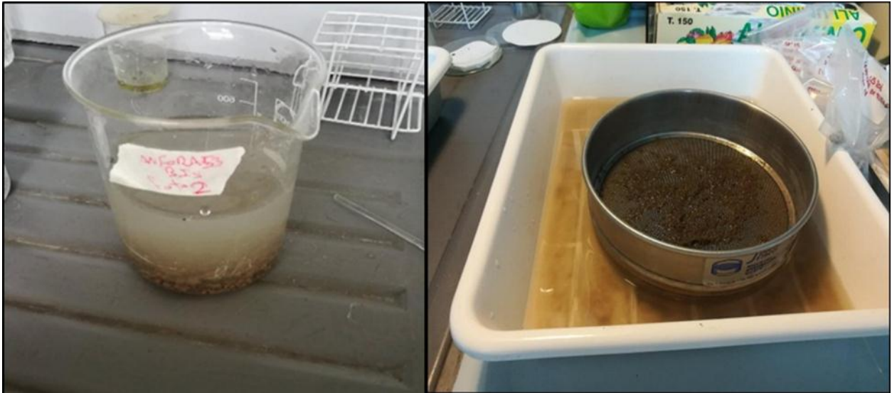
Figure 12: The treatment of the samples with water and oxygen peroxide (H 2 O 2 ), and wet sieving
