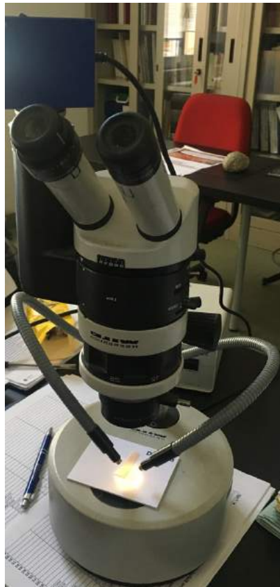
Figure 15: WILD M5A stereo microscope, coupled with led lights and ZEISS Axiocam ERc 5s camera.
