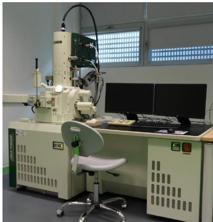
Figure 17: SEM-EDS system. ( www.phy.uniri.hr )
