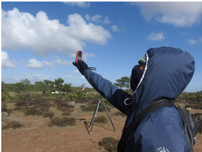
Figure 5: Example of wind speed sampling in Cabranosa (Sagres). A similar procedure was used in field data sampling at BSJWF in 2007.
