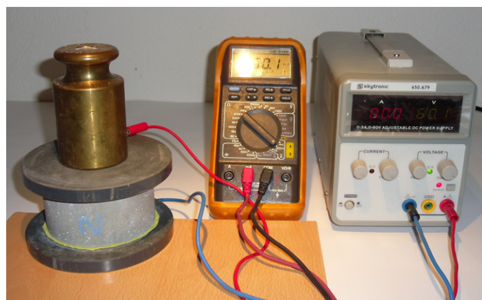
Figure 3. (a) Chloride migration test assembly scheme. (b) Electrical resistivity setup
