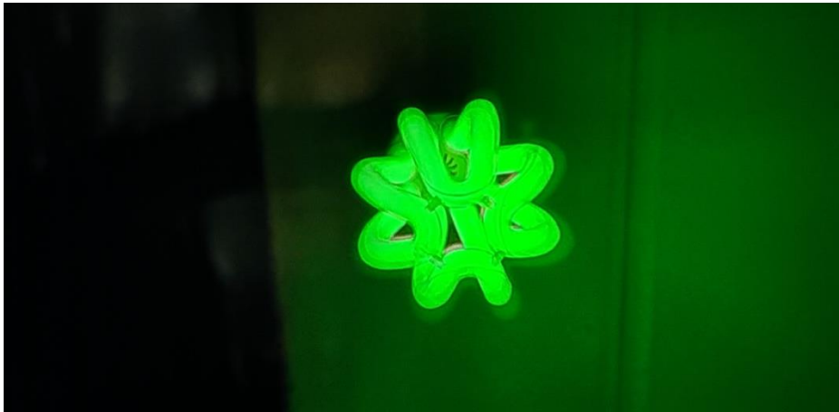
Figure 4.15: Photograph of the second image (Image 2 in Fig. 4.13), viewed at an angle with respect to the holographic plate. In this case, the green image of the object produced by the holographic mirror is totally separated from the partial reflection of the object in the glass, since it does not obey the ordinary laws of geometric optics with respect to the plane defined by the glass plate.
