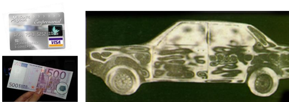
Figure 2.3: Holograms used as security elements in documents - credit cards, banknotes and in quality control. (e.g. measurement of small deformations in the automobile industry).
