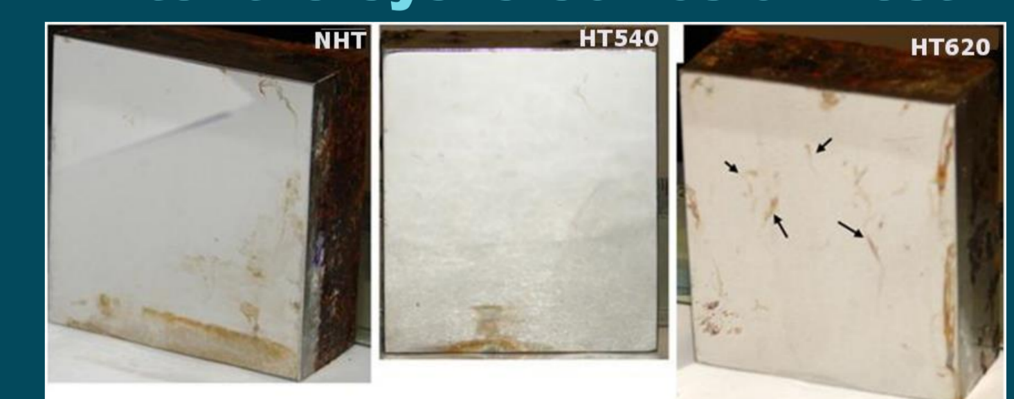
After the Cyclic Corrosion Test
