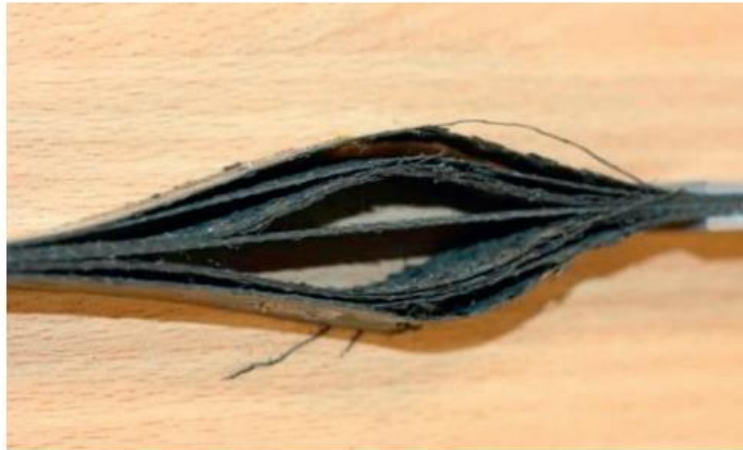
Figure 52 - Delamination during tensile test due to differences of stiffness of plies - (Jollivet, Peyrac e Lefebvre 2013)
