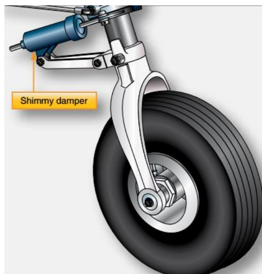
Figure 20 - Shimmy damper device - Oleo-Pneumatic Landing gear leg - (FAA - Federal Aviation Administration s.d.)
