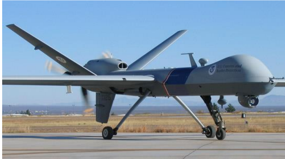
Figure 16 - MQ9 Reaper aircraft with a composite landing gear - (Fiber Dynamics s.d.)
