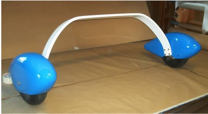
Figure 6 - Light Aircraft glass fiber composite main landing gear - (C. Composites s.d.)
