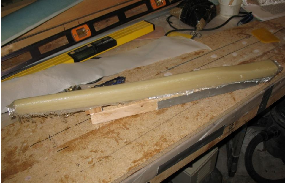
Figure 27 - Construction of a composite Landing Gear strut of a Varieze type aircraft - (Wade s.d.)
