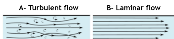
Figure 14 - Flow regimes (A) turbulent flow; (B) laminar flow [93].
