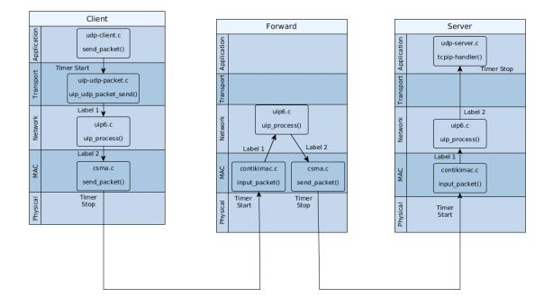
Figure 3.2: Contiki network stack scope
