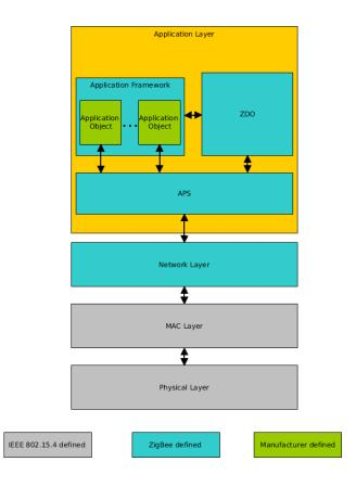
Figure 2.4: ZigBee Stack Architecture
