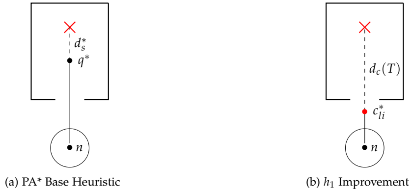
Figure 4.1: Impact of using the distance to the critical point, d_c(T) , as the guaranteed minimum perception distance on the improved heuristic h_1 .
