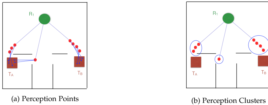
Figure 7.2: a) When running PA* from the robot initial position to each point inside target regions, the search returns an optimal perception point, shown as a red dot; b) in order to reduce the number of possible combinations, the perception points are clustered in groups as single waypoints for path planning.
