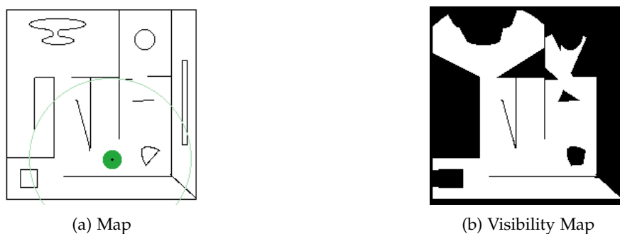
Figure 2.4: a) A simulated map of obstacles in black, a circular robot in green, and the robot sensing range in light green; b) the Visibility Map, with regions that can be sensed by the robot in white and occluded regions in black.
