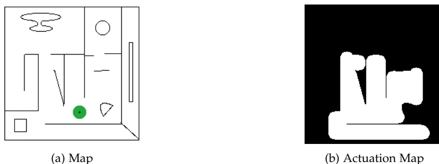
Figure 2.2: a) A simulated map with obstacles in black and a circular robot in green; b) the resulting actuation map, with regions that can be covered by the robot in white and regions that cannot be covered by the robot in black, assuming the actuation range is equal to the robot size.
