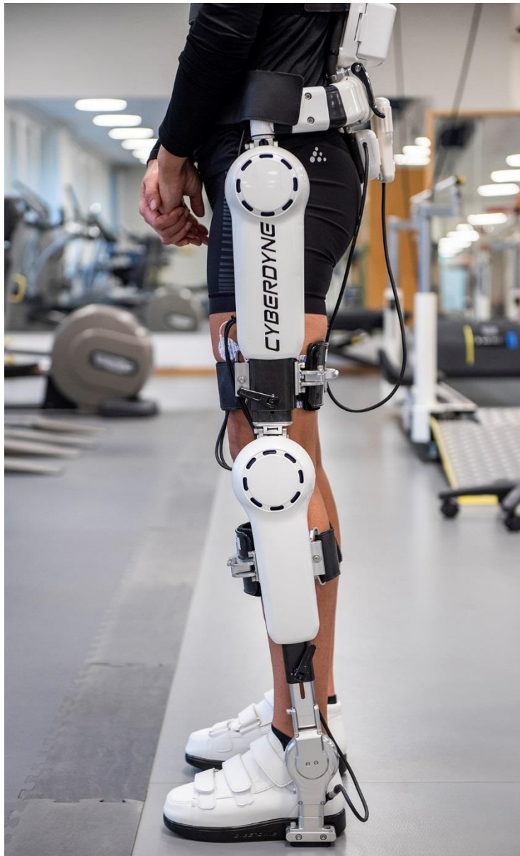
Figure 3. Single leg version of the Hybrid Assistive Limb (HAL). Photo by: Johan Adelgren
