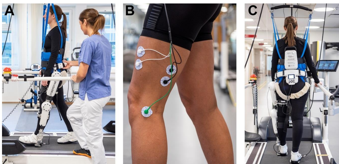
Figure 5. A+C) Illustration of HAL training, performed on a treadmill with body weight support. B) Surface electromyography (EMG) to capture the wearer's voluntary muscle activation. EMG-electrodes were affixed over the following muscles: biceps femoris (knee flexion), quadriceps vastus lateralis (knee extension) (in picture) and rectus femoris (hip flexion), gluteus maximus (hip extension) (not in picture). A reference electrode was placed over the lateral femur condyle. Photos by: Johan Adelgren
