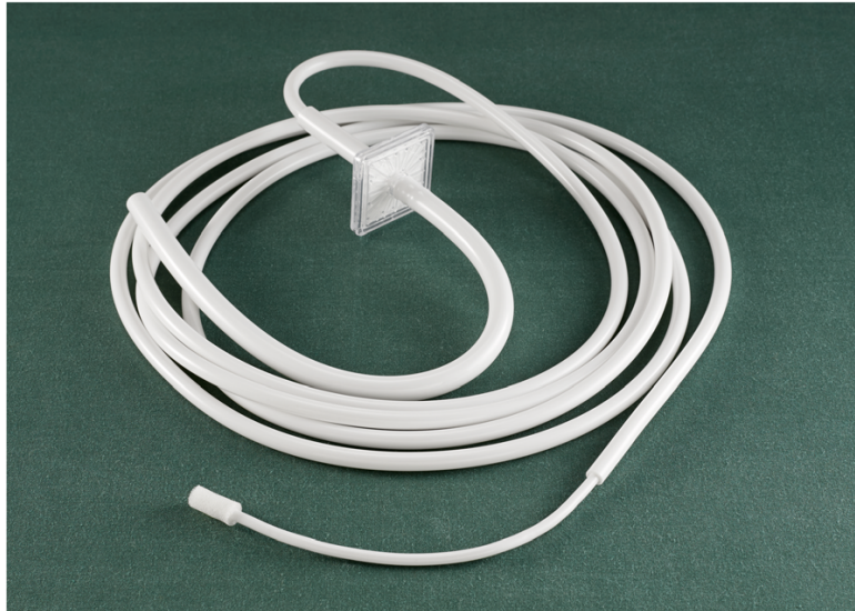
FIGURE 3. The mini CO 2 -diffuser (CarbonMini® Cardia Innovation AB, Stockholm, Sweden), is a single-use insufflation device that consists of three parts, a two m long PVC tube, a bacterial filter, a 0.20 m PVC tube that has an inner diameter of 1 mm inside which a metal thread runs, and a cylindrical diffuser consisting of soft polyurethane (approx. 4 cm 2 ).
