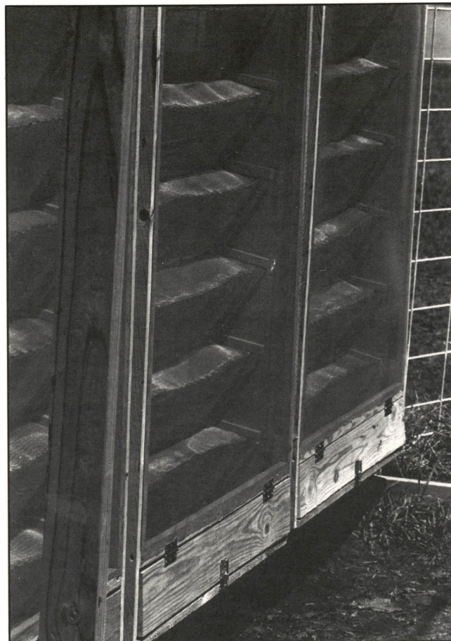
Figure 1. The trapping elements are in place, as viewed from the side. These elements are held into the framing with screw hooks and eyes and can be removed for maintenance.
