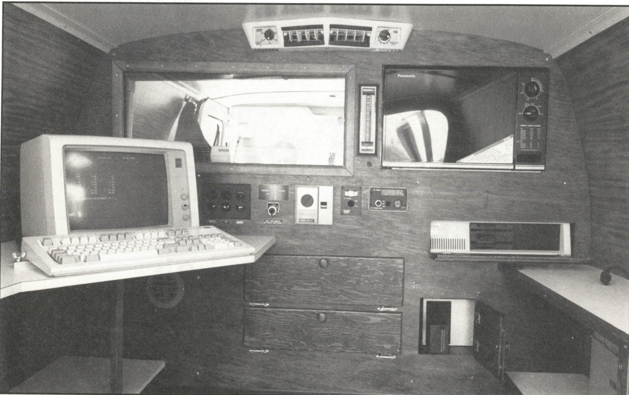
The NIR van contains all the necessities for testing forage quality, including a microwave oven for drying samples, an NIR forage analyzer, and a microcomputer which compares sample's results against conventionally tested samples.
