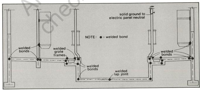
Bonding as defined in the National Electrical Code means the permanent joining together of metallic parts to form an electrically conductive path, which will assure electrical continuity and the capacity to conduct safely any current likely to be present.
