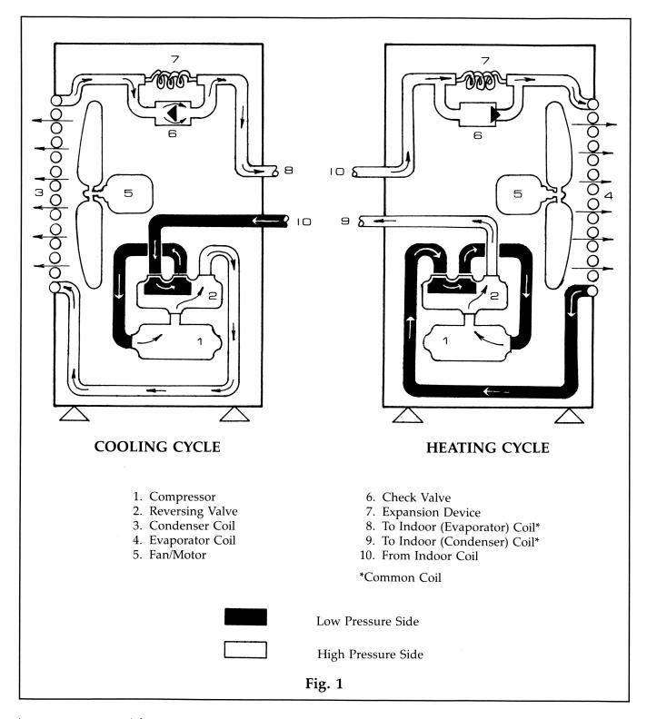
ing environment. A heat pump uses energy only to run the fan and compressor motors.
