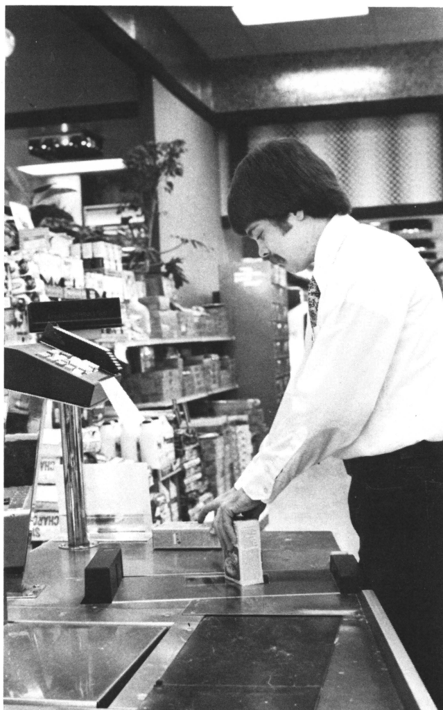
As the product is placed on the machine's scanner, a computer identifies the UPC and the price is flashed on the register.
