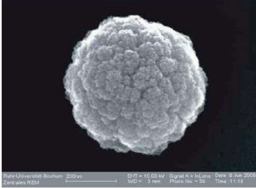
Figure 2.13: Often carbonaceous nano-particles grown in discharges have a cauliflower-like surface indicating a porous structure. From [29];
