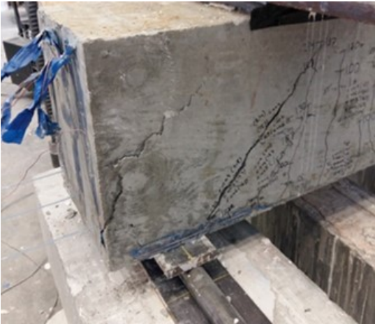
Figure 3.5 Side-face blowout failure – Specimen H-3-8-5-13-F4.1-2
