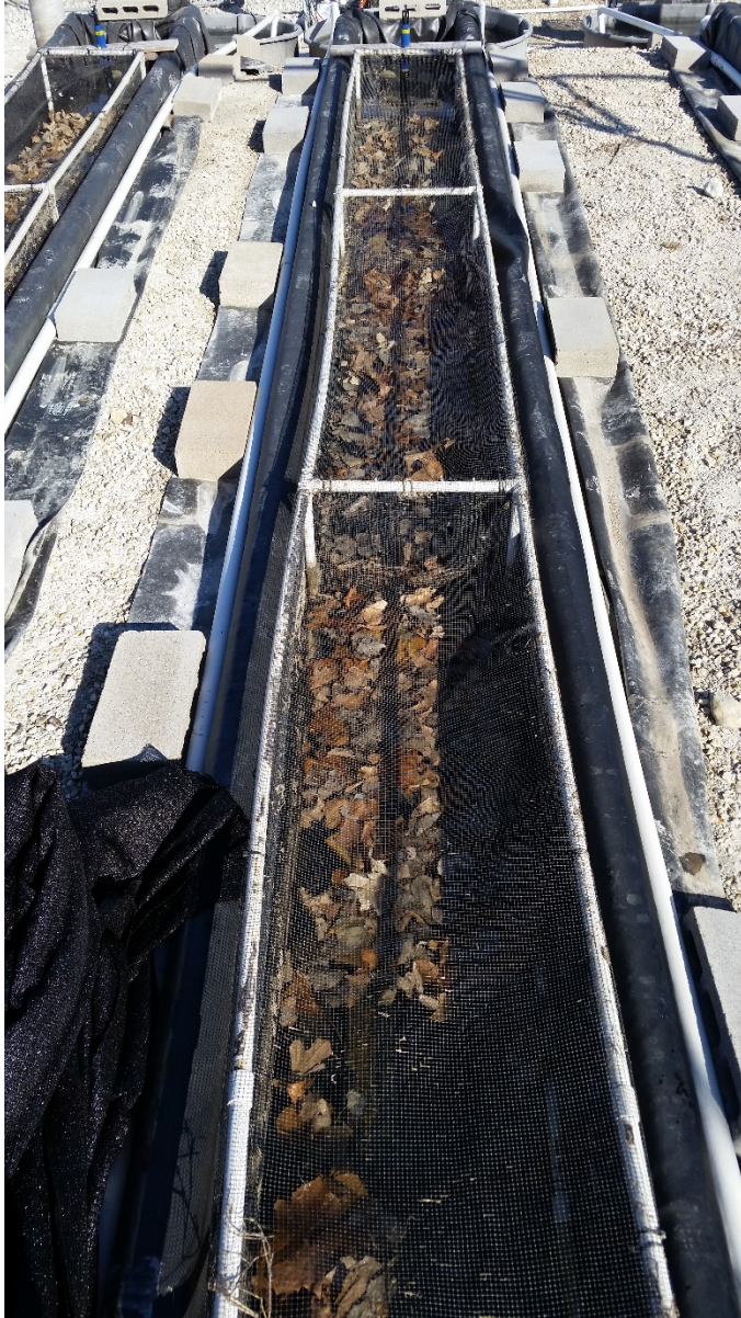
Figure S4. Looking downstream at the glide section immediately after placement of litter in the three glide cages.
