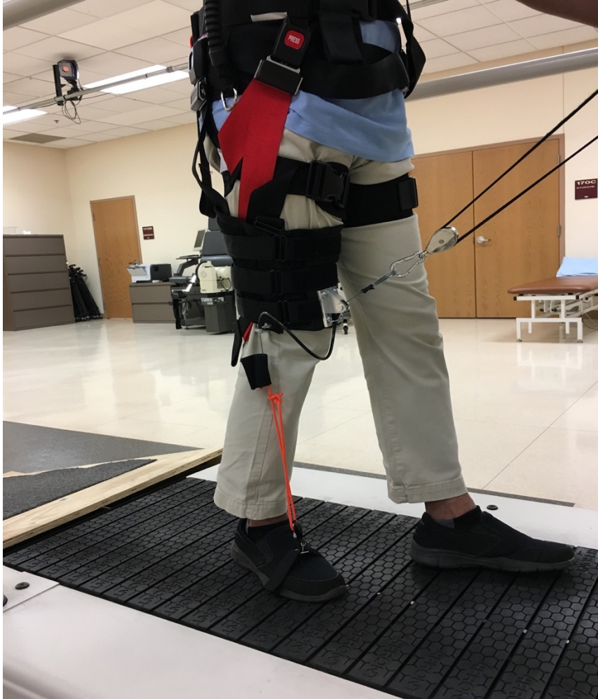
Figure 1: The assistive device used to assist the participants in hip flexion and ankle dorsiflexion at the swing phase of a gait cycle on the affected side.
