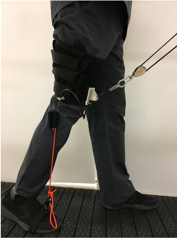
Figure 1: The assistive walking device which helps the participants in hip flexion and ankle dorsiflexion during swing phase of gait cycle in the affected lower limb.
