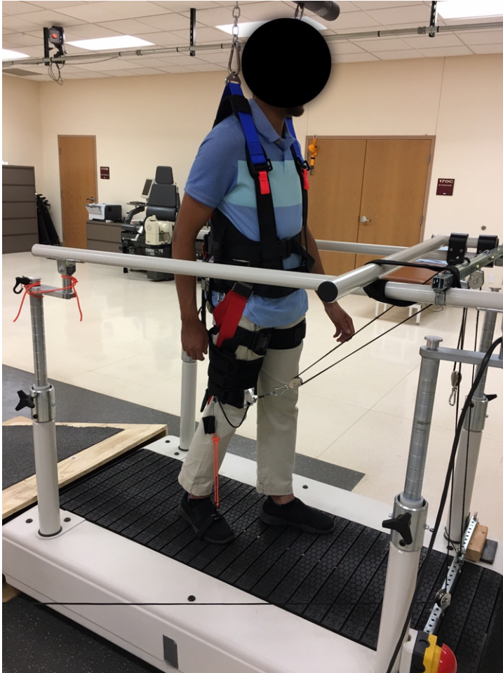
Figure 1: The assistive device used to assist the participants in hip flexion and ankle dorsiflexion at the swing phase of a gait cycle on the affected side.
