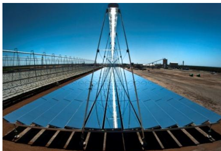
Figure 7. Schematic view of a typical LFR power system.
