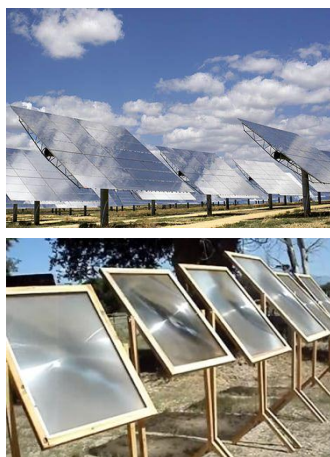
Figure. 2. Solar mirrors (upper) and solar lenses (lower) which both concentrate solar radiation.
