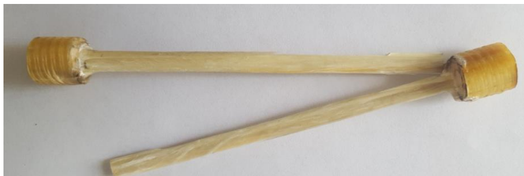
Figure 3.5. - Fracture of a glass fiber plastic sample
