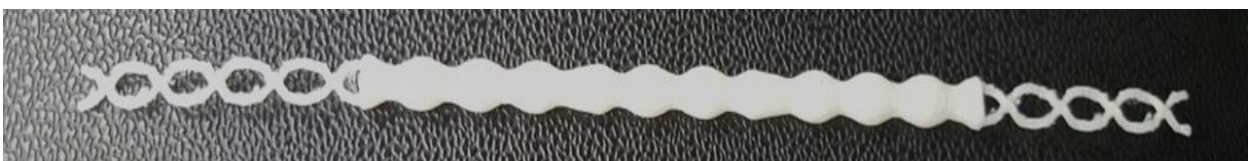
Figure 5.3. -Prototype of the rod printed on the 3D printer Mojo
