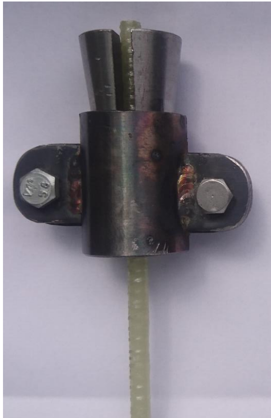
Figure 5.11. - Prototype terminal clamp for testing and obtaining prestressed composite reinforcement with periodic profile
