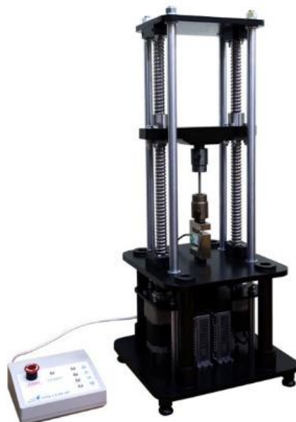
Figure 3.1. - Educational testing machine NTC-13.04.20 "Tearing machine 20kN"
