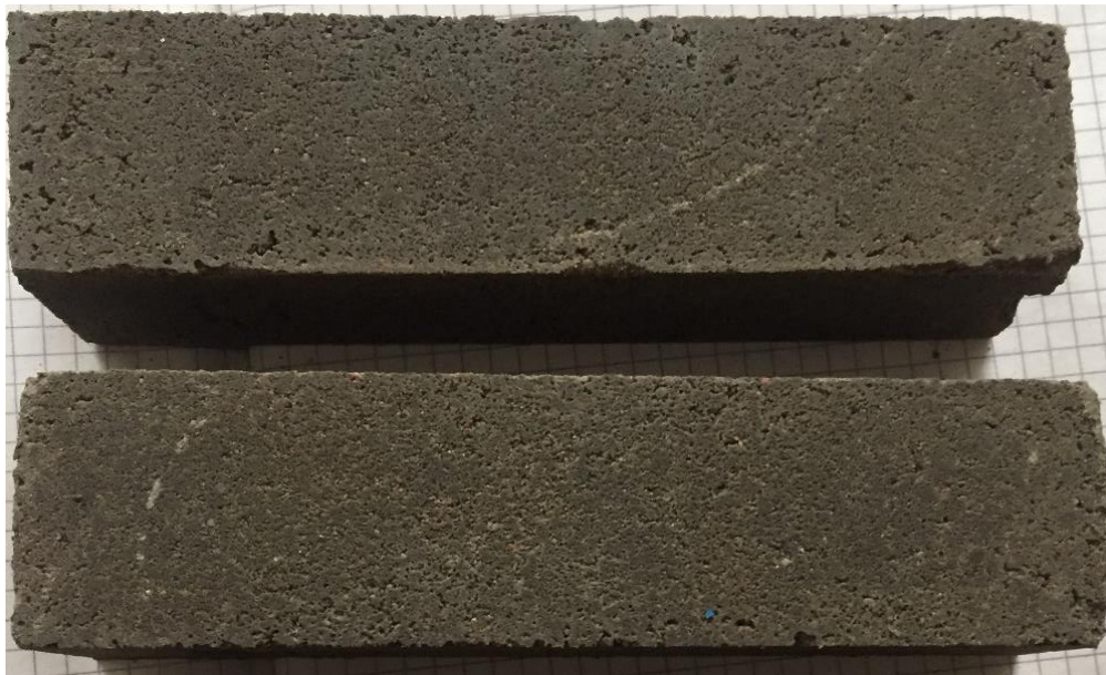
Figure 4.4. – The samples-beams based on the complex binder
