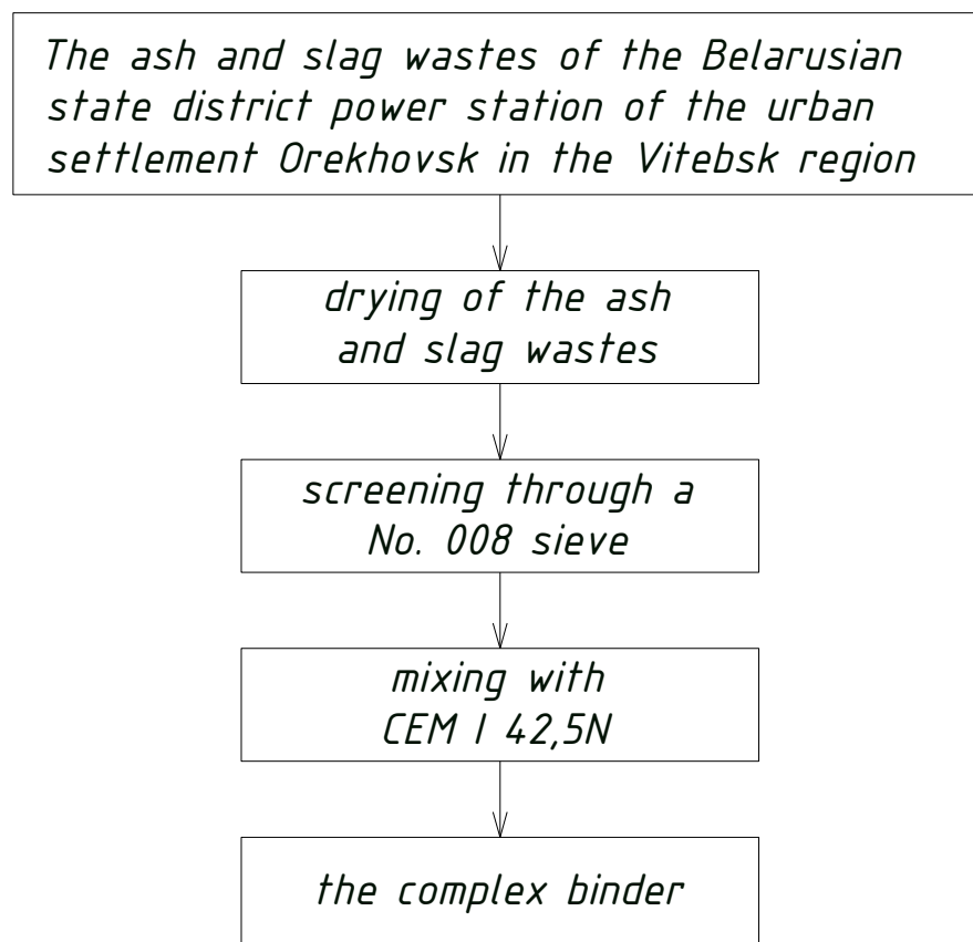
Figure 3.1. – Preparation of the complex binder
