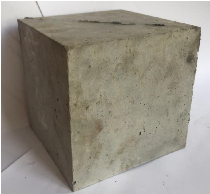
Figure 4.7. – The sample of concrete on the complex binder
