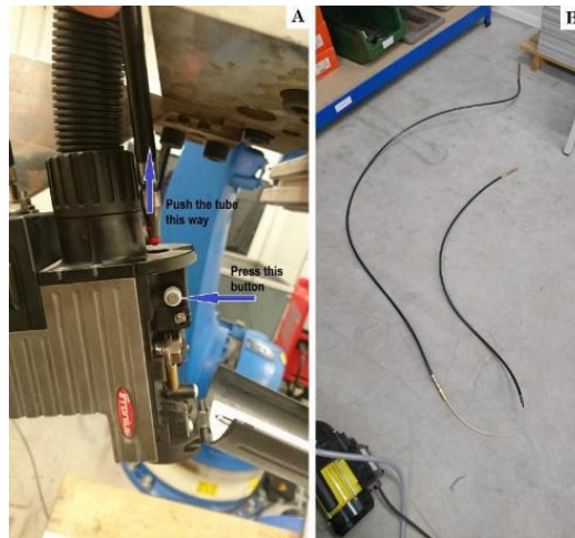
Figure B.19 – A-In the torch remove the tube, too; B- After the tubes are out
