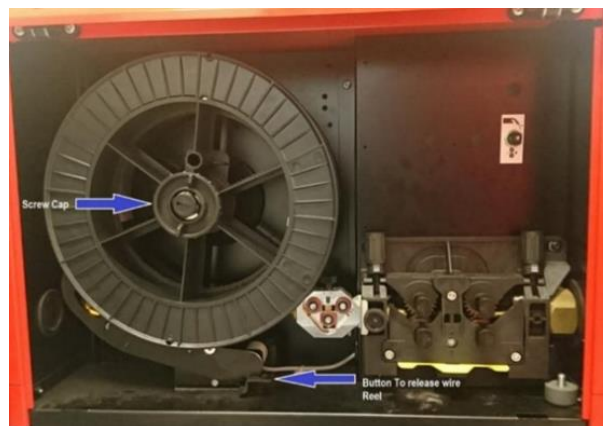
Figure B.9 – Press the button in the bottom and untighten the holder (plastic tight cap)
