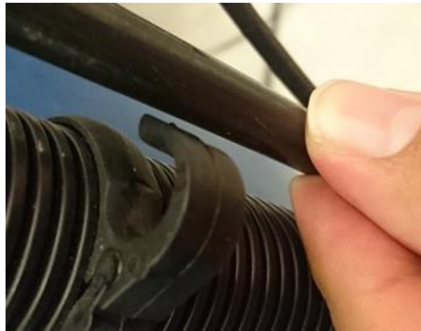
Figure B.17 – Loose the tube from the main tube
