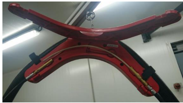
Figure B.33 – Open the buffer so you can see if the wire reaches it
