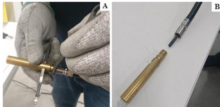
Figure B.20 – A-Detach the tubes end (yellow) from the tube (black); B-The interior has to be removed
