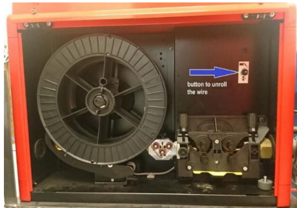
Figure B.34 – Press the button to unroll the wire until it gets to the buffer
