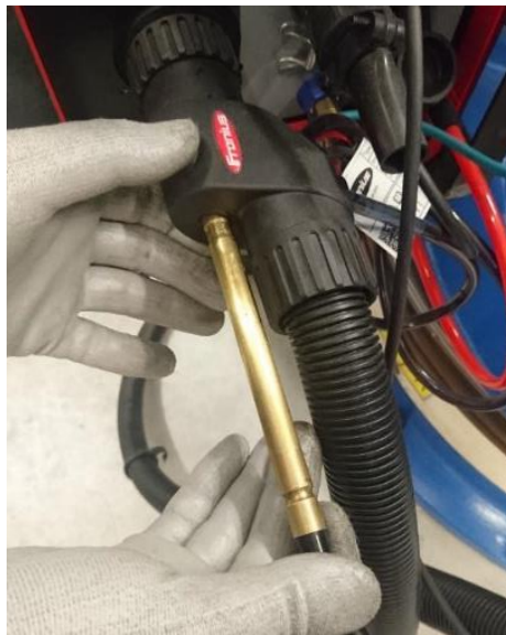
Figure B.23 – After they are both changed, put the tubes back in place
