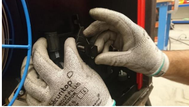
Figure B.25 – It is important to change all the four rollers
