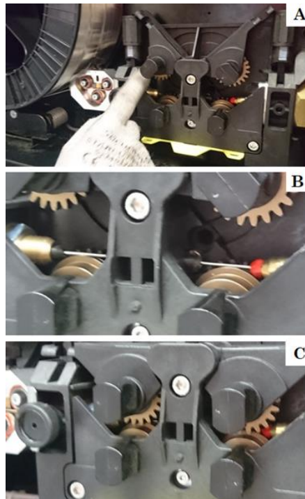
Figure B.31 – A-Open the roller holder's so the wire can be passed through; B- Through the tip into the tube; C- Close the roller's holders and adjust them if needed
