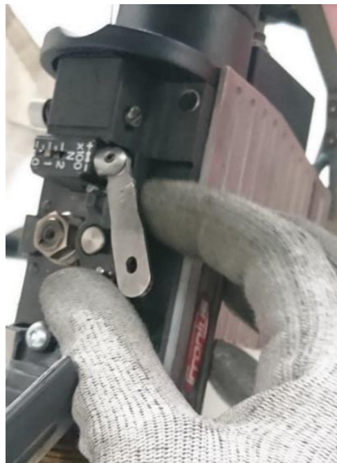
Figure B.39 – Detach the roller holder on the Torch, as seen in the photo below. The roller must be open to let the wire pass through
