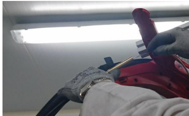
Figure B.36 – Pass the wire through the yellow tube and into the black one, which leads to the nozzle
