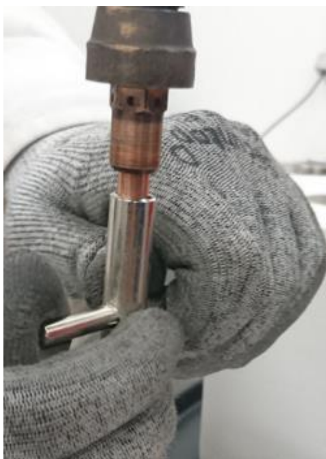
Figure B.43 – Untighten the nozzle in the torch
