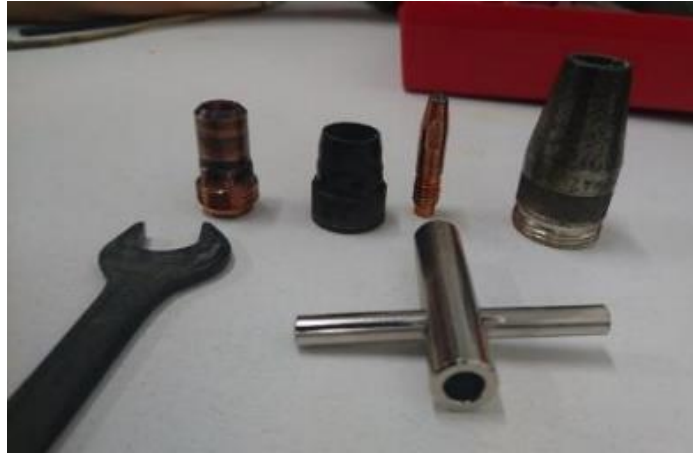
Figure B.45 – Parts that form the nozzle, and tools needed to disassemble them
