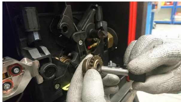
Figure B.24 – This procedure consists in taking the spindle out. The roller pops off
