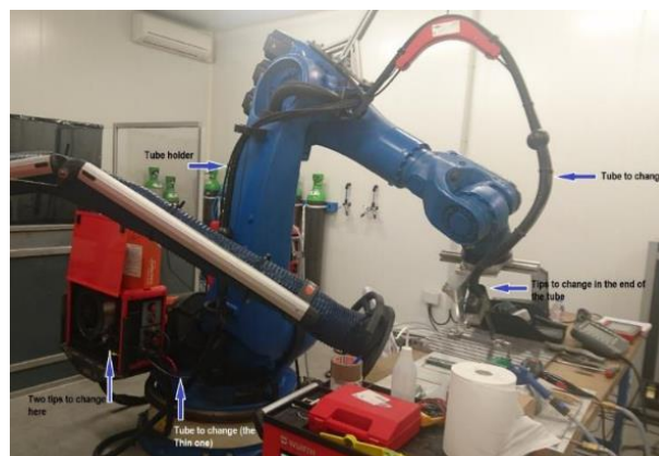
Figure B.12 - Location of the tubes and tips
