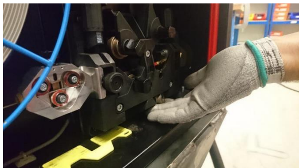
Figure B.28 – Put the bottom rollers under the black plastic
