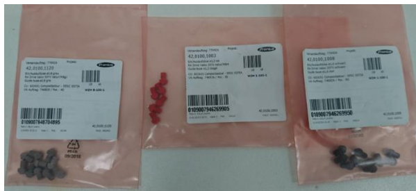
Figure B.11 – Different size tips to be attached in the black tubes according to each size of wire
