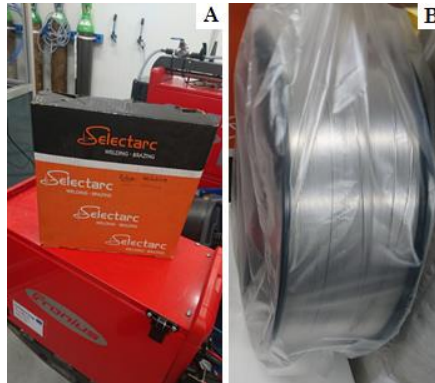
Figure B.29 – Unpack a new wire from the box that comes in a spool
