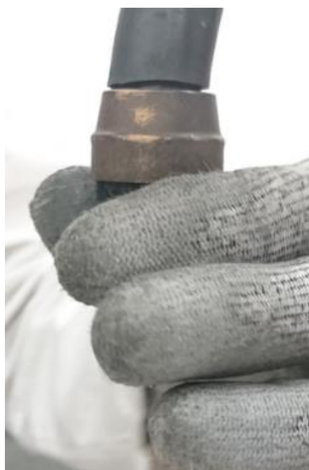
Figure B.44 – Untighten the nozzles cover
