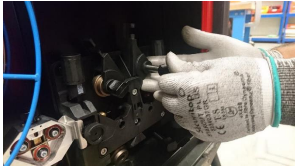
Figure B.26 – Put the upper rollers through the top
