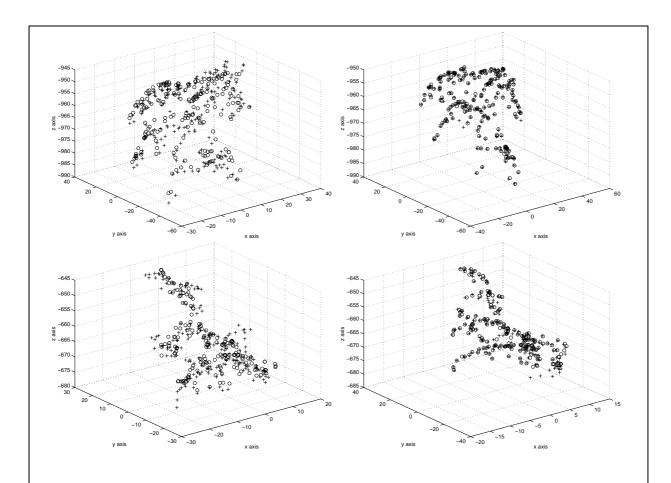
Figure 5: The results for the matching of 200 randomly selected points with uniform distribution from the bird1 and bunny1 images respectively by the k-GA algorithm. Left column: Before registration, Right column: after registration. Top row: bird1-2; bottom row: bunny1-2.
