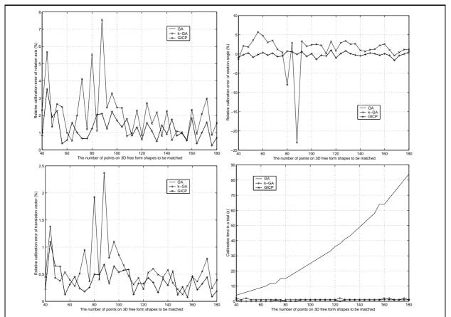
Figure 3: The relative calibration errors of the parameters of interest and calibration time as a function of the number of points on the 3D free form shapes to be matched. Top left: rotation axis; Top right: rotation angle; Bottom left: translation vector; Bottom right: the time in seconds for matching in a trial.
