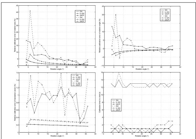
Figure 2: The relative calibration errors of the parameters of interest and calibration time as a function of the rotation angle. Top left: rotation axis; Top right: rotation angle; Bottom left: translation vector; Bottom right: the time in seconds for matching in a trial.
