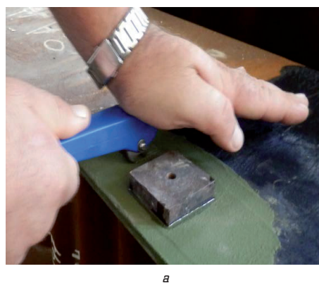
Fig. 2. Thickness measurements of metal plastic film and protective coating using NOVOTEST CT-1 device
