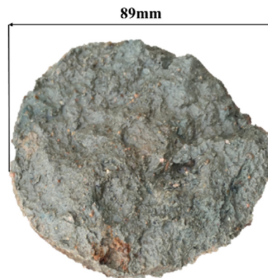
Fig. 18. Photograph of the core sample at 2 m depth in the field test area.
