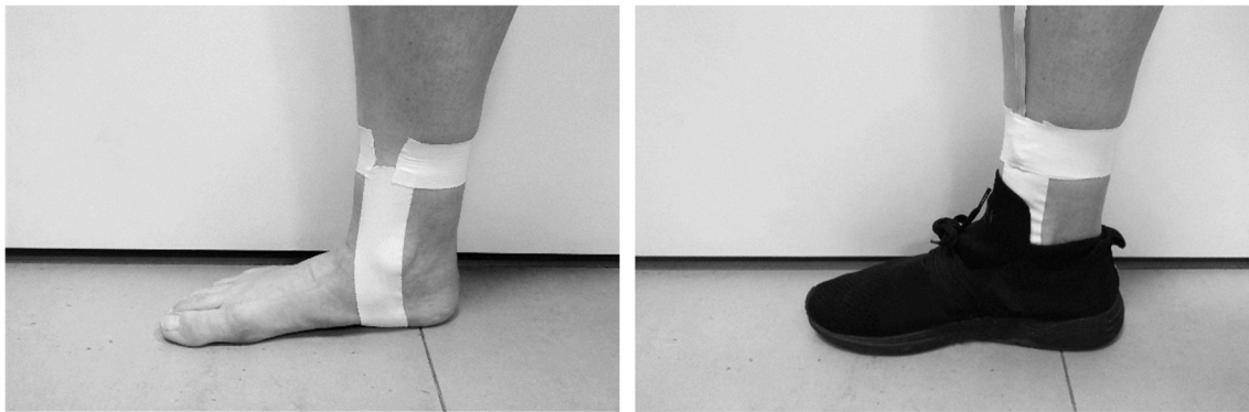
Figure 2. Attachment method of the sensor to the lower leg. (left) Pretension is applied to the skin near the site of attachment. (right) The accelerometer is firmly fixed with tape.
